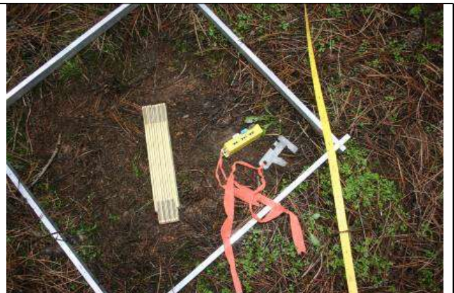
Figure 7. Linear sampling with combined recording using a “go-no-go” device
