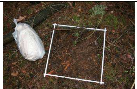
Figure 5. Square sampling with a 1 square meter grid
